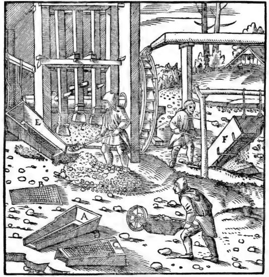
A—Box laid flat on the ground. B—Its bottom which is made of iron wire. C—Box inverted. D—Iron rods. E—Box suspended from a beam, the inside being visible.
